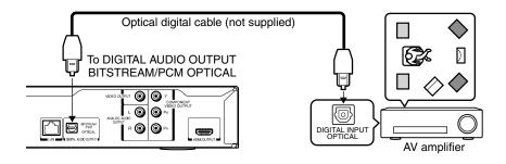
\*To use the optical digital output, use an optical cable to connect this jack to an optical audio input on a device capable of processing Dolby Digital, DTS bitstream, or PCM audio.
